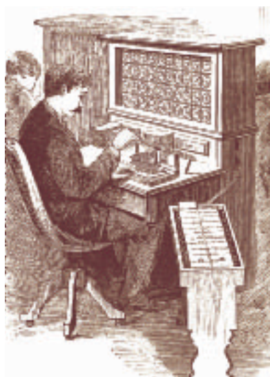
▲ The Electric Tabulating Machine processed the 1890 census in 2½ years, a job that would have taken nearly 10 years to complete by hand.
